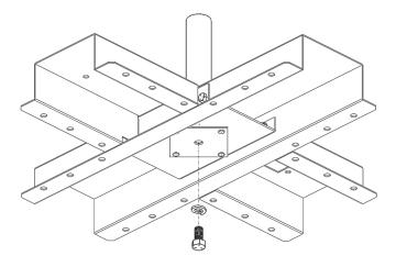
**5)** Tighten hardware from <u>step 2</u> using 1/2" or 13mm wrench.
