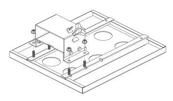
1) Slide your assembled Pallet and Pallet Arm onto Rotor Arm.
