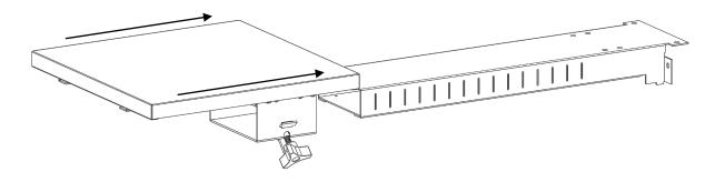
**3)** Tighten knob on Pallet Arm. Do not over tighten.
