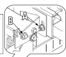
To Adjust Screen angle Front to Back. Loosen (2) Bolts (Marked B) Slightly and Set Screen Level.
