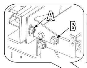
To Adjust Screen Height and angle Left to Right. Loosen (1) Nut (Marked A) Slightly and Set Screen Level. Adjust one side at a time.
