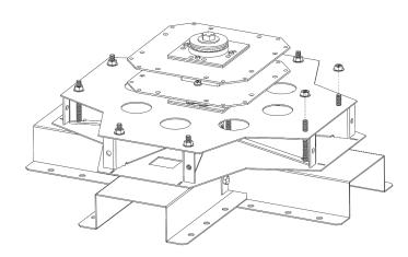
3) Align Rotor Arm with Bolts in Rotor Hub. Tabs on bottom of Rotor Arm drop into slots in Bottom Rotor Hub Plate.
