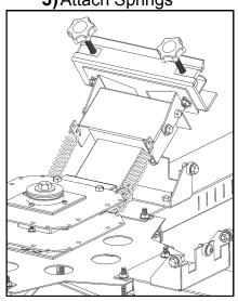
4) Install Stop Bar as shown. Stop Bar must be installed while head is in the Down position.
